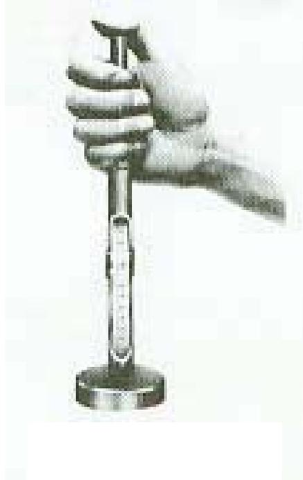
**Gambar 10.3** Mesin uji kekerasan Shore scleroscope.
