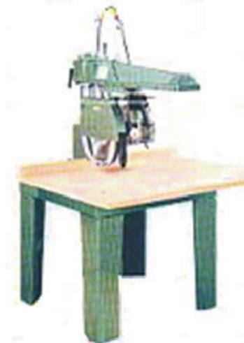
**Gambar 11.2** Radial Arm Saw
