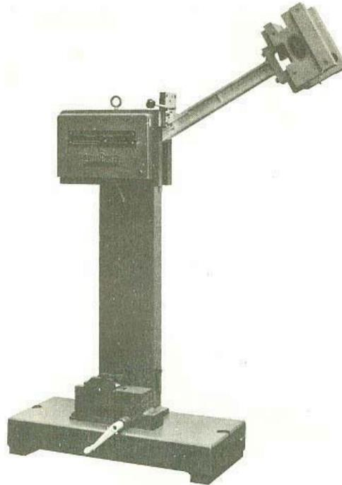
**Gambar 10.48** Mesin uji pukul takik (Impact Testing Machine)
