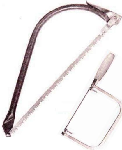
**Gambar 11.20** Gergaji tangan (Handsaws) type busur (Bowsaw)
