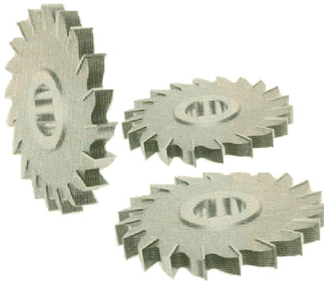
**Gambar 9.82** *Side face end mill cutter*
