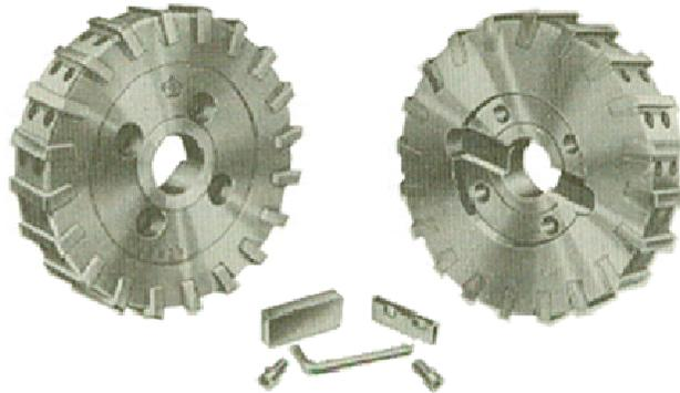
**Gambar 9.81** Face mill cutter
